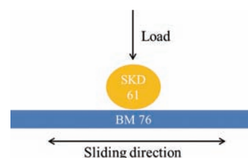
Figure 2. Pin-on-disc type of reciprocating friction wear test.
